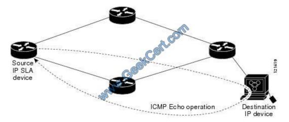
The IP SLAs ICMP Echo operation conforms to the same IETF specifications for ICMP ping testing and the two methods result in the same response times. Configuring a Basic ICMP Echo Operation on the Source Device SUMMARY STEPS
