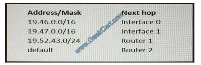
Refer to the exhibit. Which next hop will the router select if given an IP packet with the destination address 19.48.254.3?
