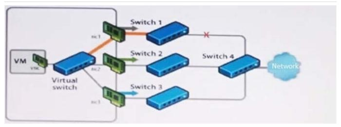
Each ESXi host has three NICs assigned to a virtual switch.
