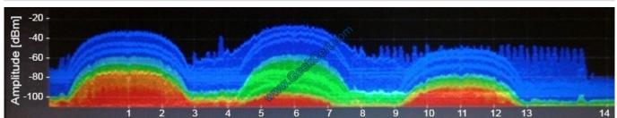
An engineer is troubleshooting non-802.11 interference and observes this output. Which type of interference signatures can be identified?
