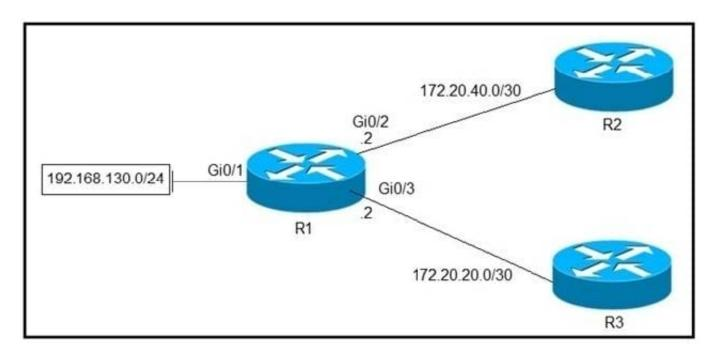
A. access-list 1 permit 192.168.130.0 0.0.0.255! interface Gi0/2 ip policy route-map test! route-map test permit 10 match ip address 1 set ip next-hop 172.20.20.2
