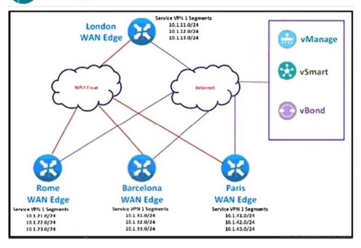
The SD-WAN network is configured with a default full-mesh topology. An engineer wants Barcelona and Paris to communicate to each other through the London site using a control policy. Which control policy configuration accomplishes the task?
