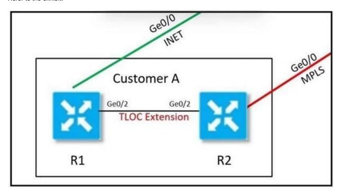
An MPLS connection on R2 must extend to R1 Users behind R1 must have dual connectivity for data traffic Which configuration provides R1 control connectivity over the MPLS connection?
