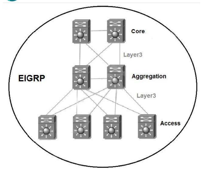
The full EIGRP routing table is advertised throughout the network. Currently, users experience data loss when any one link in the network fails. An architect must optimize the network to reduce the impact when a link fails. Which solution should the architect include in the design?
