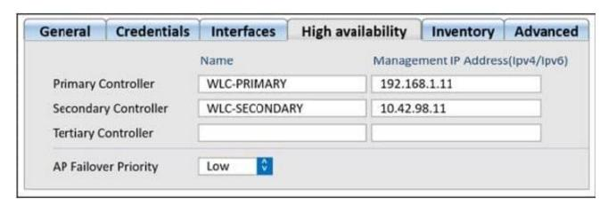
A network engineer has identified that during a recent controller failure, several APs failed over to the tertiary controller instead of the secondary controller. The configuration from one of the APs is provided. Which design consideration led to the issue?
