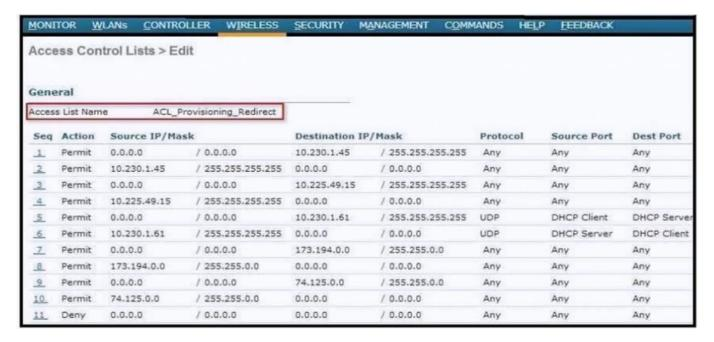
An ACL is configured to restrict access for BYOD clients. The ACL must redirect devices to the guest portal. To which two devices on the local network must the ACL allow access other than the DHCP server? (Choose two.)
