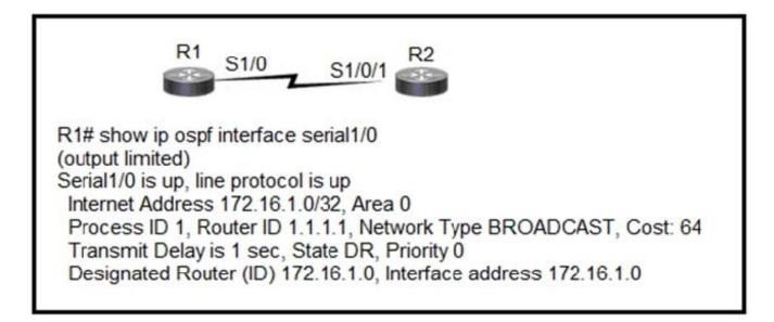
While configuring router 2 with all the default values, a network engineer cannot see any route received in router 1. How should the engineer solve the issue?
