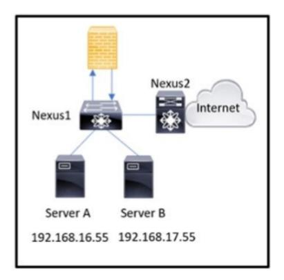
The Cisco Nexus Series Switch with hostname Nexus1 is the default gateway for server A and server B. Both servers must have reachability to the internet, however, server A internet traffic must pass through the firewall for deep packet inspection. Also, the firewall must inspect any communication between server A and server B.
