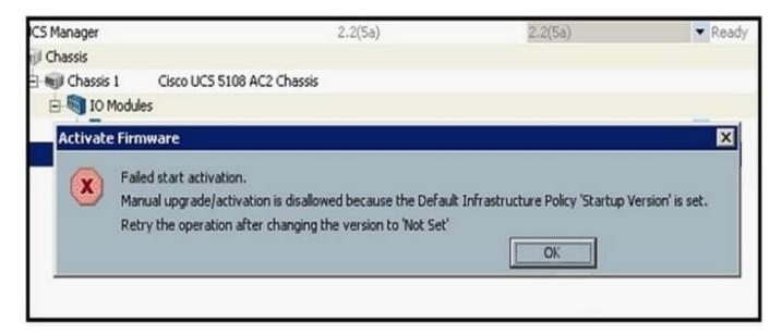
Cisco UCS Manager is being upgraded using the Auto Install feature, but the FSM fails. Which action resolves the issue?
