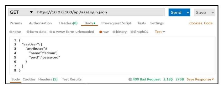
A Postman call to a Cisco APIC fails. The access credentials were confirmed to be configured as expected. Which action resolves the issue?
