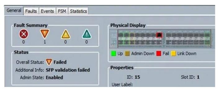
When an engineer inserts 8-Gb Fibre Channel SFP port 15 on a Cisco UCS Fabric Interconnect, the port fails. What is causing this issue?
