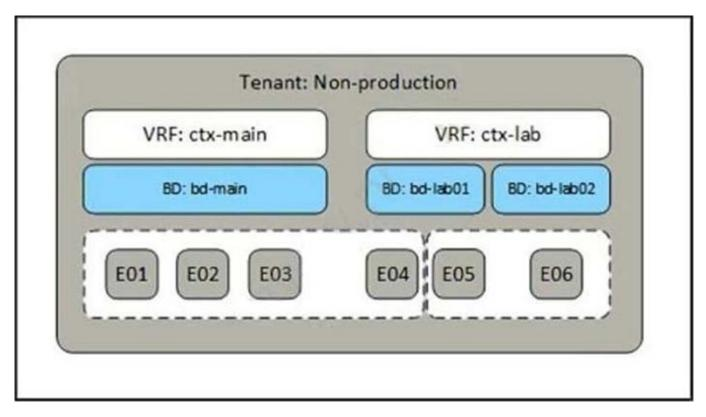
A network engineer must complete the Cisco ACI implementation based on the logical system design created by the systems architect. Which Cisco ACI object is required where the dotted line indicates to complete the task?
