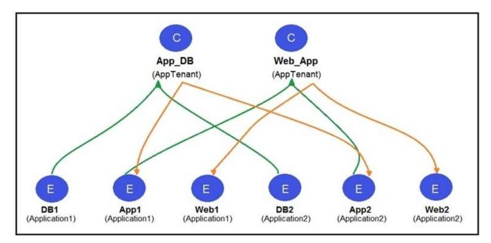
Refer to the exhibit. Two application profiles are configured in the same tenant and different VRFs. Which contract scope is configured to allow communication between the two application profiles?
