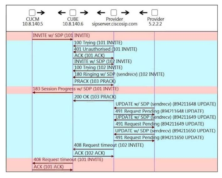
A Cisco Unified Border Element continues to send 180/183 with the required: 100rel header to Cisco UCM, and the call
