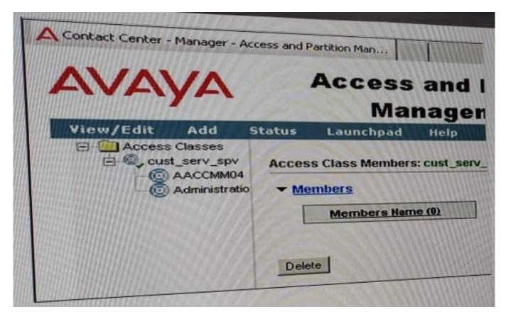
The graphic shows an Access Class, cust\_serv\_spv, and the two components that comprise the Access Class definition, the contact Center Manager Server (CCMS) AACCMM04, and the Administration. Permissions levels ate granted to items within the launchpad through the creation of an Access Class.
