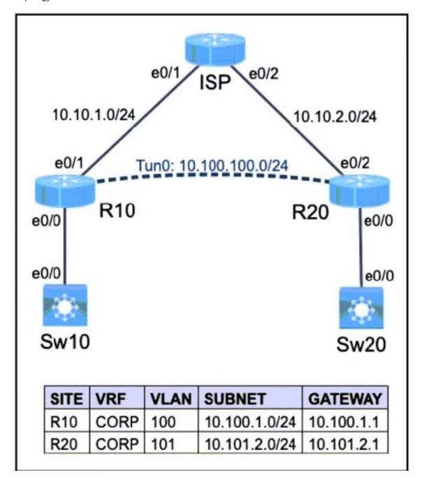
The operations team started configuring network devices for a new site. R10 and R20 are preconfigured with the CORP VRF. R10 has network connectivity to R20. Complete the configurations to achieve these goals:
