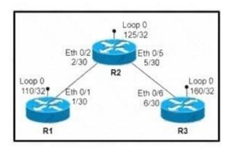
An engineer configures routing between all routers and must build a configuration to connect R1 to R3 via a GRE tunnel Which configuration must be applied?
