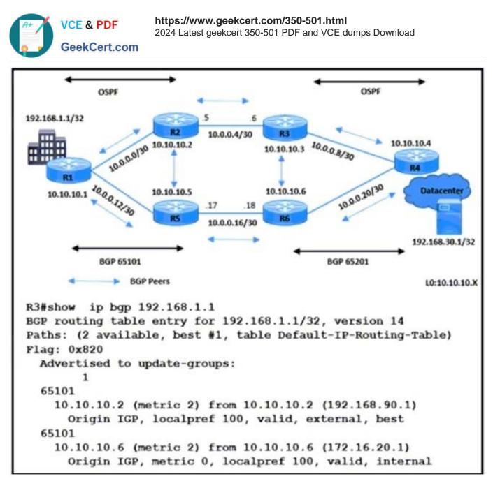
Refer to the exhibit. All BGP peering in AS 65101 and 65201 is enabled. The operations team is told that traffic destined to 192.168.1.1/32 from R4 does not use the path R3-R2-R1 as expected. An engineer debugs the issue and determines that 192.168.1.1/32 is advertised in the BGP routing table on R1. Which action resolves the issue?
