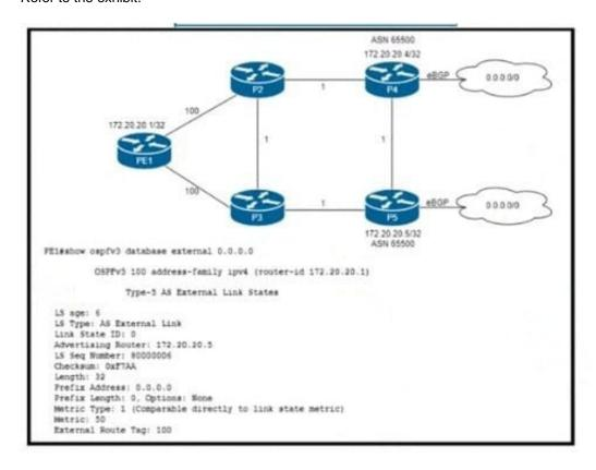
Router P4 and P5 receive the 0.0.0.0/0 route from the ISP via eBGP peering P4 is the primary Internet gateway router, and P5 is its Backup. P5 is already advertising a default route into OSPF domain. Which configuration must Be applied to P4 so that advertises a default route Into OSPF and Becomes me primary internet gateway for the network?
