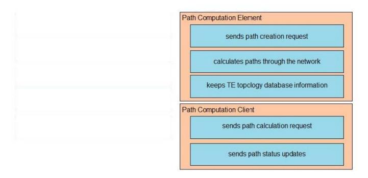
Path Computation Element (Calculates paths through the network, keeps TE topology database information, sends path status updates) Path computation Client (sends path calculation request, sends path creation request)
