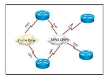
An enterprise is migrating its single-area OSPF network from a Frame Relay WAN service to an MPLS L3VPN service. Frame Relay will remain in only a few sites that require increased resiliency via two different WAN connections.
