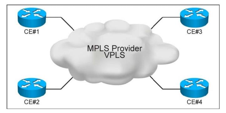
Four customer sites are connected through an EoMPLS-based VPLS over an MPLS provider. You are migrating from OSPF to multi-level IS-IS as the routing protocol to run on the four CE routers, and connectivity between all four sites is required. You want to control which CE or CEs will be elected as the Designated Intermediate System. Which two key aspects should be taken into account? (Choose two.)
