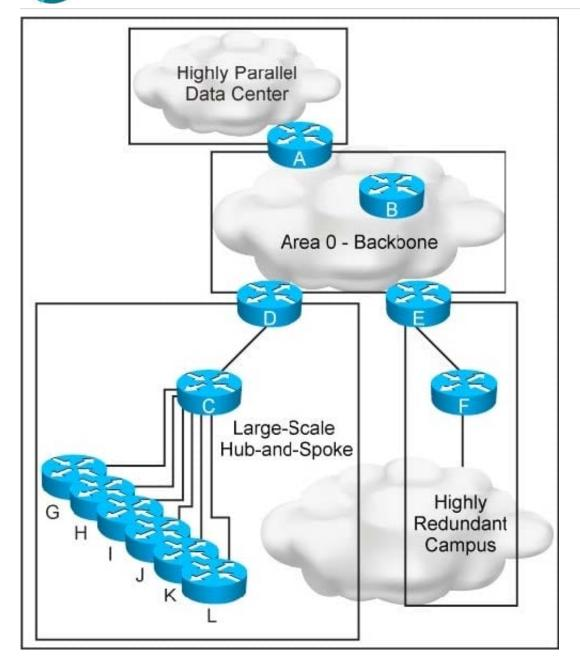
This new OSPF network has four areas, but the hub-and-spoke area experiences frequent flapping. In order to fix this design failure, which two mechanisms can you use to isolate the data center area from the hub-and-spoke area without losing Ip connectivity? (Choose two)
