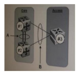
Virtual Link Aggregation Control Protocol (VLACP) is configured by port, and traffic is only forwarded across the uplinks when VLCAP is up and running correctly.
