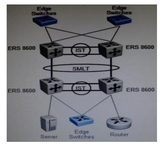
A campus network has been established with four Ethernet Routing Switch (ERS) 8600 switches in a switch cluster, two pairs with an Inter Switch Trunks (IST) running Split Multi Link Trunk (SMLT) and Routed Split Multi-Link Trunking (RSMLT). The traffic filters are required to block specific source IP addresses to be forwarded through the core.
