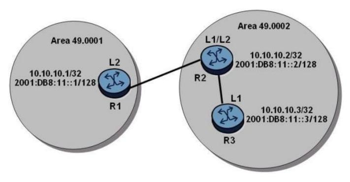
The routers have an established IS-IS L2 adjacency on which IPv4 system addresses are exchanged. An operator successfully configures multi-topology IS-IS routing so that the IPv6 system addresses are also exchanged between routers.
