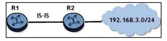
Router 2 advertises the network 192.168.3.0/24 to router R1 via IS-IS. How can router R1 ensure that it discards the route?
