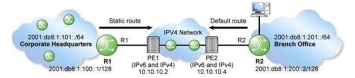
A service provider is deploying a 6 over 4 tunnel to connect a customer\\'s corporate IPv6 network to all devices at the branch office as shown in the exhibit. Which command is used to create the route to the branch office network on PE1?
