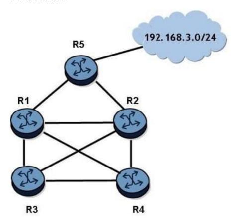
OSPF is operational on all links in the network diagram, all routers are the same cost, and all routers are configured with an ECMP value of 4. Router R5 advertises the prefix 192.168.3.0/24 into OSPF.
