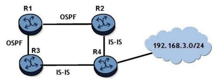
If router R2 re-distributes the IS-IS route 192.168.3.0/24 into OSPF, router R3 will receive two routes to 192.168.3.0/24. Assume that all IS-IS routers are L1/L2 capable and are in the same area.
