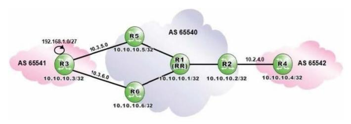
Router R1 is a route reflector with clients R2, R5 and R6. Router R3 advertises the prefix 192.168.1.0/27 to routers R5 and R6. Assuming that routers R1, R2 and R4 are configured with "add-paths ipv4 send 2 receive", what is the expected output of "show router bgp routes" when executed on router R2?
