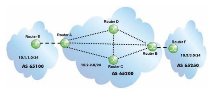
After router A receives the BGP update for the 10.3.3.0/24 prefix, which routers will the route be propagated to?
