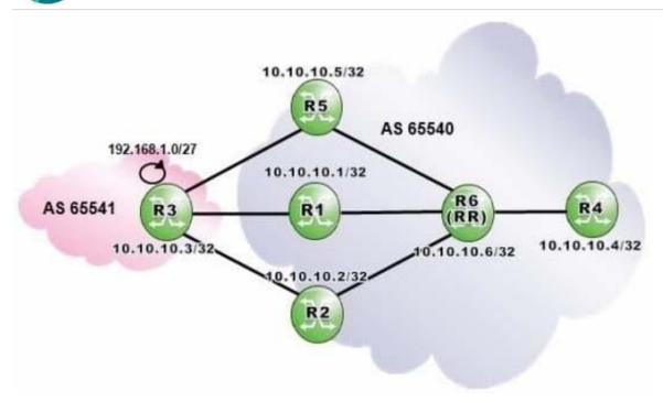
Router R6 is a route reflector with clients R1, R2, R4 and R5. R4 receives three routes from router R6 and is configured with ECMP 3. Given the following BGP configuration on router R4, how many primary and backup paths will be present in router R4\\'s BGP routing table?
