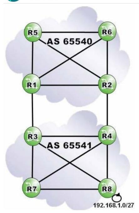
Router R2 receives a route to 192.168.1.0/27 from router R4, and sets the local preference to 110. Router R1 receives a route to 192.168.1.0/27 from router R3, and sets the local preference to 80. Both ASs have a full iBGP mesh.
