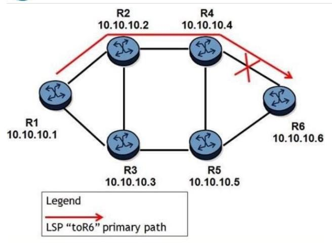
An LSP path is established on router R1 toward router R6. After router R4 detects that the link between routers R4 and R6 goes down, which of the following will affect the failure propagation time?
