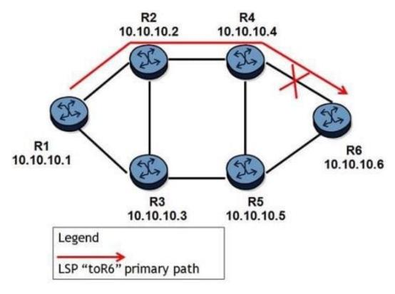
An LSP path is established on router R1 toward router R6. If the link between routers R4 and R6 goes down, which of the following is the quickest way for service recovery?
