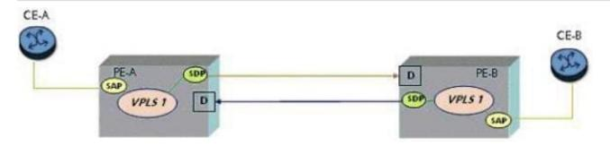
The SAP on PE-A has been configured with dot1q encapsulation. The SAP on PE-B has been configured with qinq encapsulation. CE-A sends frames with a single tag of 100. The VLAN tag from CE-A must be passed transparently. CE-B is expecting a frame with a top tag of 200 and bottom tag of 100. Which of the following is the correct SAP id for PE-B?
