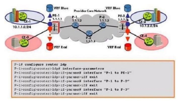
An Alcatel-Lucent 7750 SR is to be configured as a core router that supports VPRNs using LDP as the transport protocol. Which of the following best describes this configuration?
