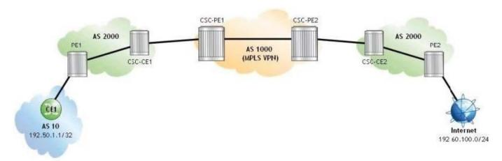
A Carrier Supporting Carrier (CSC) VPRN is configured on an Alcatel-Lucent 7750 SR for a customer carrier who is an Internet Service Provider (ISP). Which of the following configuration steps is NOT required?
