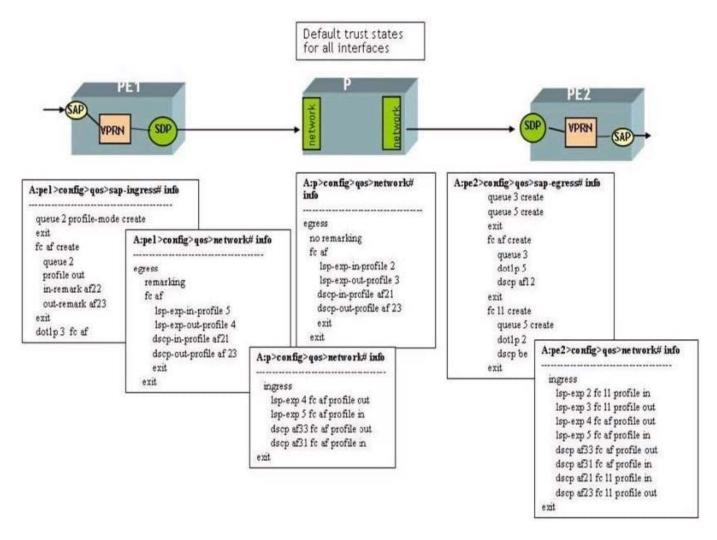
All interfaces are using their default trust states and MPLS is used as the transport tunnel. The SAP-ingress, SAP-egress, and network QoS policies have been configured as shown below. Assume that the default network-queue policy is used on each router.
