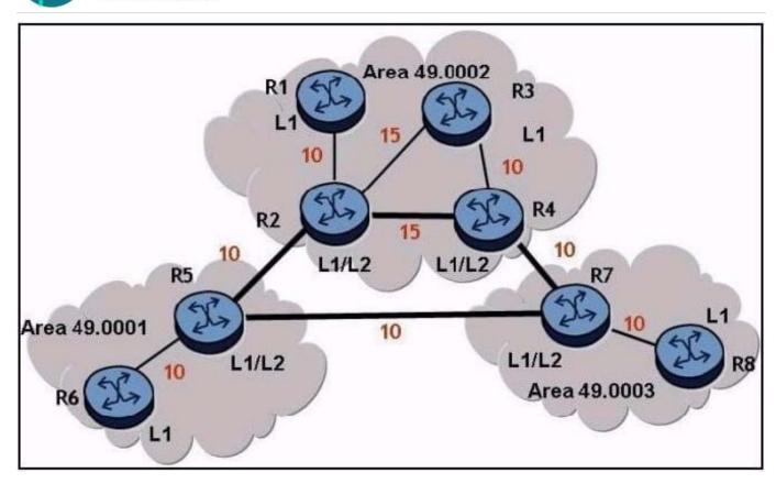
Given the diagram below, what path will traffic follow from router R6 to router R3, and from router R3 to router R6, if IS-IS is the routing protocol? The numbers beside the links are the metrics for that link.
