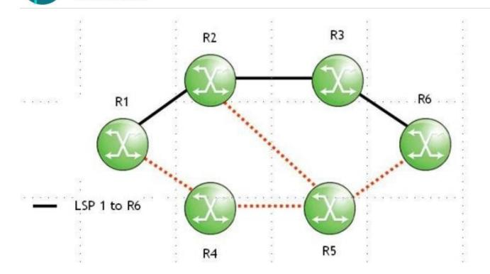
LSP 1\\'s link between routers R3 and R6 has failed, and the RESV state at router R3 has timed out. Which of the following actions will router R3 initiate?
