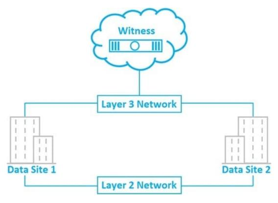
A vSAN Cluster stretched across Data Site 1 and Data Site 2 has a vSAN data network configured with an MTU of 9000. The witness node has been placed in a remote site across a WAN with an MTU of 1500. The vSAN health check, \\'vSAN: MTU check (ping with large packet size)\\', reports a failed ping.
