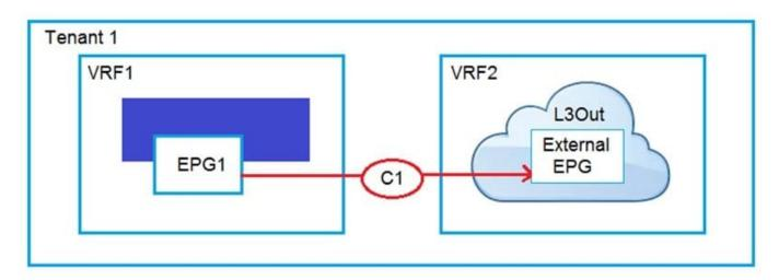
Refer to the exhibit. An engineer must have communication between EPG1 in VRF1 and External EPG in VRF2. Which three actions should be taken for the defined subnets in the L3Out External EPG to accomplish this goal? (Choose three.)
