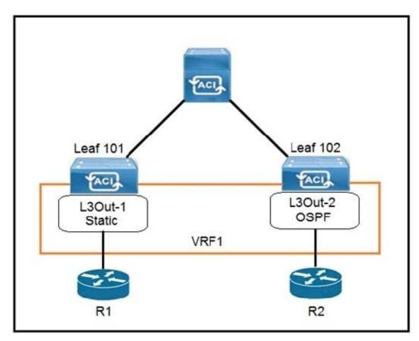
Refer to the exhibit. The 0.0.0.0/0 is configured as a default static route on L3Out-1. Which action should be taken for the 0.0.0.0/0 prefix to advertise out on L3Out-2 OSPF?
