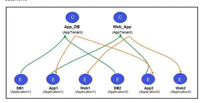
Refer to the exhibit. Two application profiles are configured in the same tenant and different VRFs. Which contract scope is configured to allow communication between the two application profiles?
