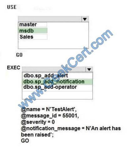
The following example adds an e-mail notification for the specified alert (Test Alert).
