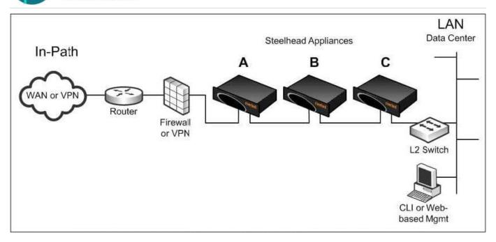
For connections initiated from the data center, there is a possibility that the Steelhead appliances shown in the exhibit will end up peering with each other, rather than the intended remote Steelhead appliances. Where are peering rules needed to prevent this problem?
