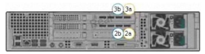
When creating a second shelf chain on a EMC Data Doman controller, what are the two recommended SAS ports that should be used?
