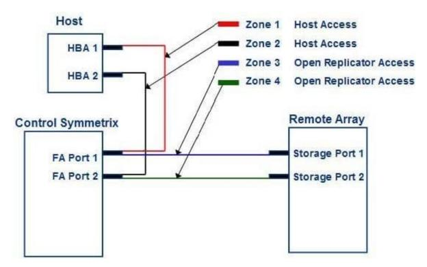
The SAN zones (Zones 3 and 4) shown in the exhibit have been created during an Open Replicator implementation. The control devices in the Symmetrix array are mapped to both front- end ports. Which Open Replicator operations can be performed?
